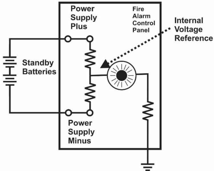
The fire alarm control panel has an Internal Voltage Reference Point. For the technician, though, finding that point on the printed circuit board is impossible. There's no test point to connect the voltmeter to, and there's no documentation to tell the technician where to find this reference point.
