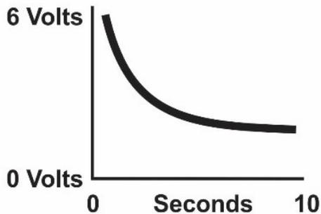
Any residual voltage between the fire alarm system and building ground is going to discharge through the voltmeter.
