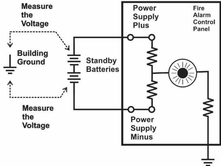
Instead trying to figure out what voltage is normal for the panel, assume that what you read is either normal, or shows ground fault. Then, when disconnecting loops to find out which loop has a ground fault, only look for a change in this voltage. If the voltage changes, you're connecting or disconnecting the ground fault. It's a troubleshooting start.
